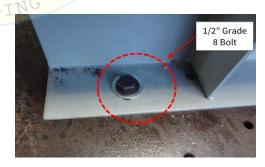
Base mounted-rigid using four (4) 1/2" -13 SAE Grade 8 bolts with lock washers and flat washers. Unit maintained structural integrity and remained functional per manufacturer requirement. Contents were included in testing per operating conditions.
