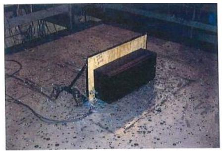
UUT wall mounted to the test fixture using five (5) #14 1" hex head type A grade 2 bolts.
