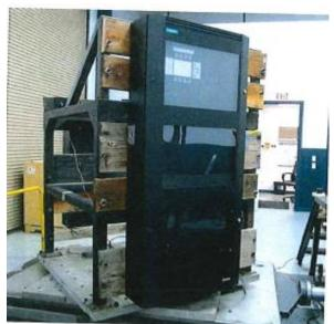
UUT wall mounted to the test fixture using six (6) 5/16" Diameter grade 8 Hex Head bolts.
