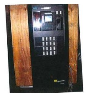
UUT wall mounted to the test fixture using six (6) #14 1" hex head type A grade 2 bolts.
