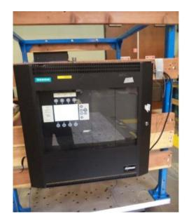
Unit was mounted to shake table wall fixture using (4) 3/8" Lag Screws.
