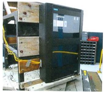
UUT wall mounted to the test fixture using four (4) 5/16" Diameter grade 8 Hex Head bolts.
