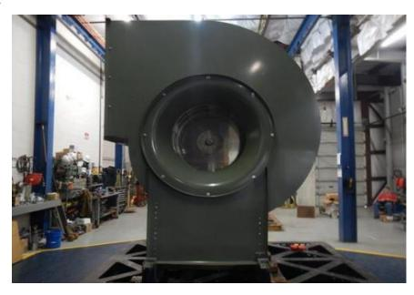
Floor mounted - isolated using (4) Mason SSLFH-C-1750 isolators w/ (1) 1/2" Grade 8 bolt attaching Isolator to unit & (2) 5/8" Grade 8 bolts attaching each isolator to the table.
