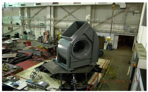
Floor mounted - isolated using (4) Caldyne Model RJJEQ 1602B style K isolators with unit mounted to 1/2" stud on top of isolators and each isolator was welded directly to the table.
