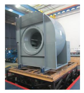
Floor mounted - isolated using (4) Mason SSLFH-C-1750 isolators w/ (1) 1/2" Grade 8 bolt attaching Isolator to unit & (2) 5/8" Grade 8 bolts attaching each isolator to the table.
