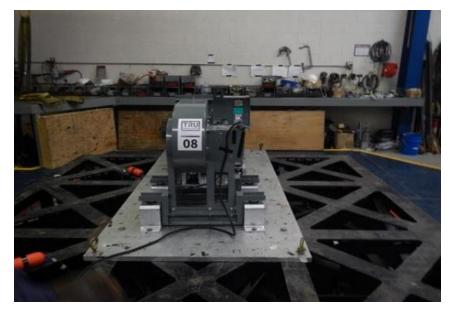
Floor mounted - isolated using (4) SRS-100 isolators w/ (1) 5/8" Grade 8 bolt attaching Isolator to unit & (2) 5/8" Grade 8 bolts attaching each isolator to the table.
