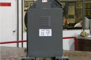
Floor mounted - isolated using (4) Caldyne Model JQA-V-E79 with unit mounted to 3/8" stud on top of isolators and each isolator was welded directly to the table.
