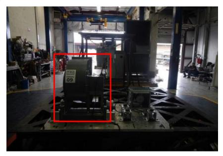
Floor mounted - isolated using (4) SRS-100 isolators w/ (1) 5/8" Grade 8 bolt attaching Isolator to unit & (2) 1/2" Grade 8 bolts attaching each isolator to the table.
