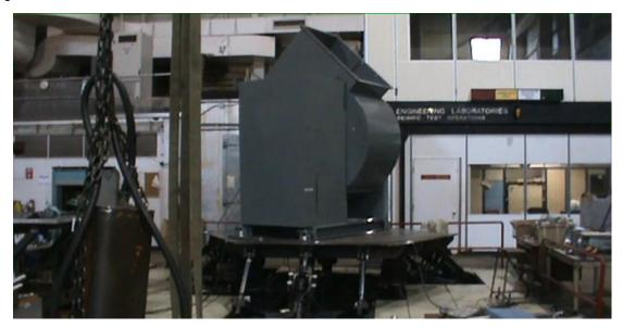
Floor mounted - isolated using (4) Caldyne Model JQB-V-E1030 isolators with unit mounted to 1/2" stud on top of isolators and (2) ½" grade 5 bolts attaching each isolator to the table.
