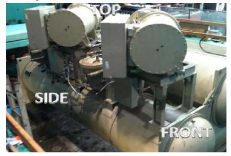
Base Mounted - Isolated on 1/4" Neoprene Pads with (8) 1" Dia. Grade 8 Bolts Unit maintained structural integrity and remained functional per manufacturer requirement. Contents were included in testing per operating conditions.
