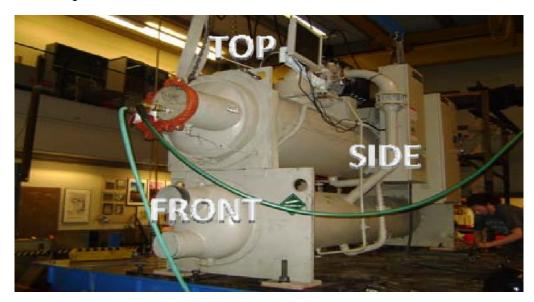
Base Mounted - Isolated on 1/4" Neoprene Pads with (8) 1" Dia. Grade 8 Bolts Unit maintained structural integrity and remained functional per manufacturer requirement. Contents were included in testing per operating conditions.
