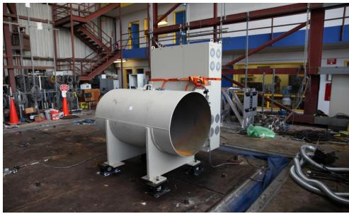
The unit was mounted on a test fixture (total wt. 3,815 lb) that was base mounted on (4) MSSH-1E-1000 isolators using (4) 5/8" diameter SAE Grade 8 bolts each to fasten the isolators to the table and (1) 3/4" SAE Grade 8 bolt each to fasten the UUT to the isolator. Unit maintained structural integrity and remained functional per manufacturer requirement.
