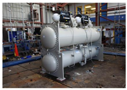
Unit was rigid base mounted to the table using (8) 1" diameter SAE Grade 8 bolts and a 1/4" ribbed neoprene pad under each mounting foot.
