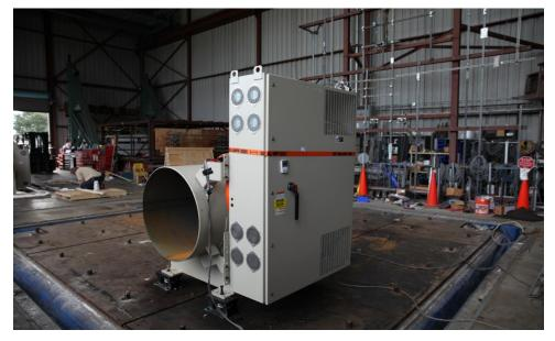
The unit was mounted on a test fixture (total wt. 3,815 lb) that was base mounted on (4) MSSH-1E-1000 isolators which were locked to simulate rigid mounting. The isolators were fastened to the table using (4) 5/8" diameter SAE Grade 8 bolts each and (1) 3/4" SAE Grade 8 bolt each to fasten the UUT to the isolator. Unit maintained structural integrity and remained functional per manufacturer requirement. Contents were included in testing per operating conditions.
