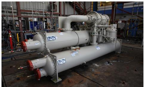
Unit was rigid base mounted to the table using (8) 1" diameter SAE Grade 8 bolts.
