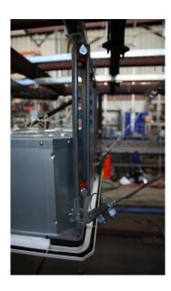
The UUT was ceiling hung using four (4) 3/8" Ø A36 hanger rods w/ rod stiffeners and four (4) 1/8" Ø diagonal cable braces w/ Mason SCB-1/SCBH-1 clips at each end. Future installations will require (8) perpendicular cable braces minimum to restrain against torsion. Unit maintained structural integrity and remained functional per manufacturer requirement. Contents were included in testing per operating conditions.
