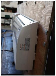
The UUT was rigid wall mounted using four (4) 3/8"A307 Thru bolts.
