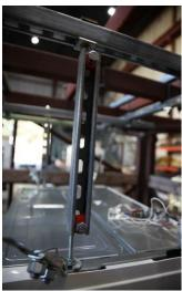
The UUT was ceiling hung using four (4) 3/8" Ø A36 hanger rods w/ rod stiffeners and four (4) 1/8" Ø diagonal cable braces w/ Mason SCB-1/SCBH-1 clips at each end.
