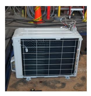
The UUT was rigid floor mounted using four (4) 3/8" lag screws with washers.
