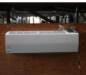
The UUT was rigid wall mounted using nine (9) #10 sheet metal screws.
