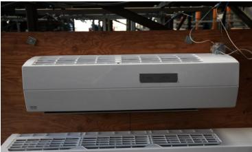
The UUT was rigid wall mounted using ten (10) #10 sheet metal screws.
