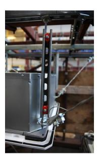
The UUT was ceiling hung using four (4) 3/8" Ø A36 hanger rods w/ rod stiffeners and four (4) 1/8" Ø diagonal cable braces w/ Mason SCB-1/SCBH-1 clips at each end. Future installations will require (8) perpendicular cable braces minimum to restrain against torsion. Unit maintained structural integrity and remained functional per manufacturer requirement. Contents were included in testing per operating conditions.
