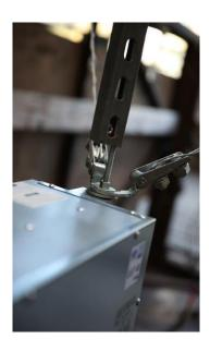
The UUT was ceiling hung using two (2) 3/8" Ø A36 hanger rods w/ rod stiffeners and four (4) 1/8" Ø diagonal cable braces w/ Mason SCB-1/SCBH-1 clips at each end.
