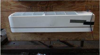
The UUT was rigid wall mounted using nineteen (19) #12 sheet metal screws.
