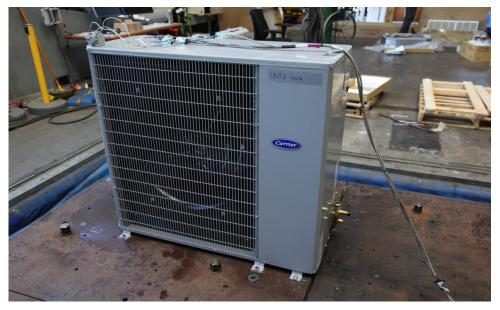
The UUT was rigid floor mounted using six (6) 3/8" Grade 8 Bolts.
