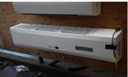
The UUT was rigid wall mounted using twenty two (22) #12 sheet metal screws.
