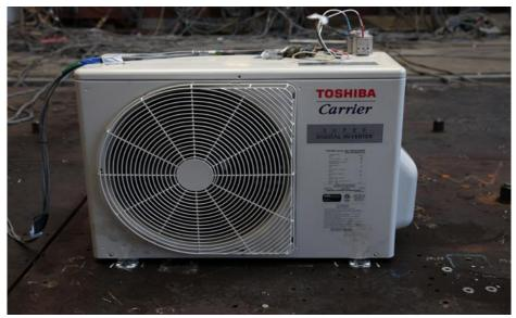
The UUT was rigid floor mounted using four (4) 3/8" Grade 8 Bolts.
