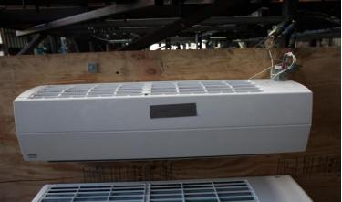
The UUT was rigid wall mounted using ten (10) #10 sheet metal screws.
