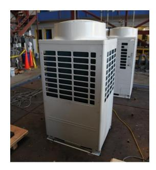
The UUT was rigid floor mounted using four (4) 1/2" A307 bolts with washers.
