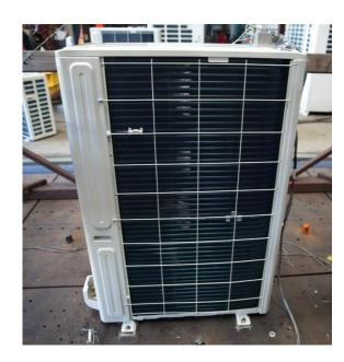
The UUT was rigid floor mounted using four (4) 3/8" A307 bolts with washers.
