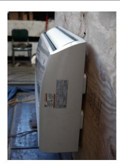
The UUT was rigid wall mounted using four (4) 3/8"A307 Thru bolts.
