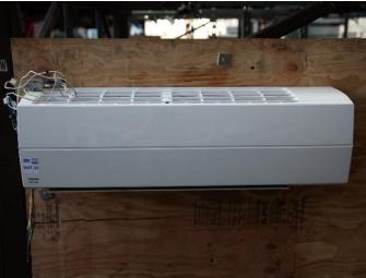
The UUT was rigid wall mounted using nine (9) #10 sheet metal screws.
