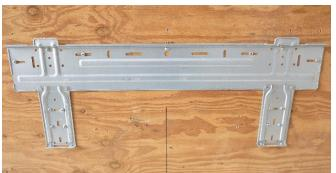
The UUT was rigid wall mounted using fifteen (15) #10 sheet metal screws.
