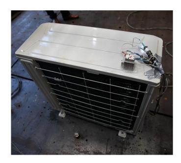
The UUT was rigid floor mounted using four (4) 3/8" A307 bolts with washers.
