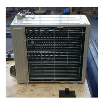
The UUT was rigid floor mounted using four (4) 3/8" lag screws with washers.
