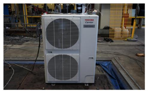
The UUT was rigid floor mounted using four (4) 1/2" Grade 8 Bolts.
