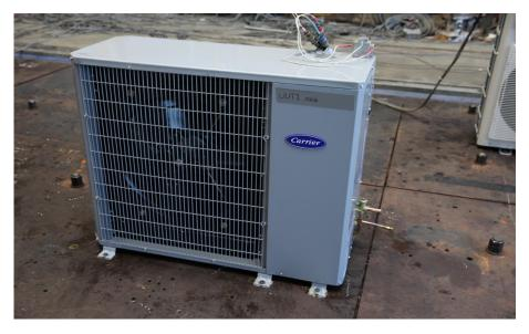
The UUT was rigid floor mounted using six (6) 3/8" Grade 8 Bolts.
