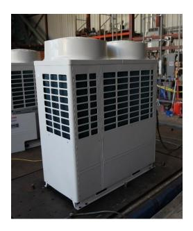
The UUT was rigid floor mounted using eight (8) 1/2" A307 bolts with washers.
