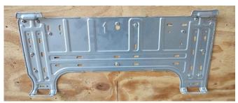
The UUT was rigid wall mounted using fifteen (15) #10 sheet metal screws.
