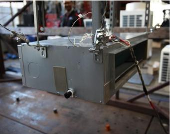
The UUT was ceiling hung using four (4) 3/8" Ø A36 hanger rods w/ rod stiffeners and four (4) 1/8" Ø diagonal cable braces w/ Mason SCB-1/SCBH-1 clips at each end.
