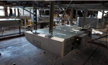
The UUT was ceiling suspended using four (4) 3/8" A36 hanger rods w/rod stiffeners & four (4) 1/8" cable braces w/Mason SCB-1/SCBH-1 clips at each end. The brackets were mounted to the unit using six (6) #10 self-tapping screws each. Unit maintained structural integrity and remained functional per manufacturer requirement. Contents were included in testing per operating conditions.
