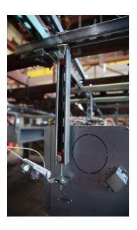
The UUT was ceiling hung using four (4) 3/8" Ø A36 hanger rods w/ rod stiffeners and four (4) 1/8" Ø diagonal cable braces w/ Mason SCB-1/SCBH-1 clips at each end.
