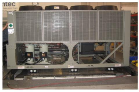
All units were filled with contents and maintained structural integrity and functionality after shake table test.
