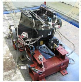
Unit mounted to the I-beams with six (6) 1/2" A307 bolts<sup>1</sup>. The GENSET rail is mounted to the shake table with with eight (8) 1/2" A307 bolts.
