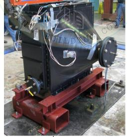
Unit mounted to the I-beams with eight (8) 1/2" A307 bolts<sup>1</sup>. The GENSET rail is mounted to the shake table with with eight (8) 1/2" A307 bolts.
