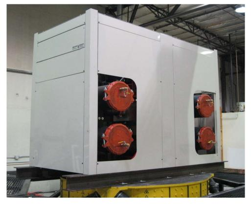
The unit was mounted to the DCL shake table interface frame with six 3/4" diameter A307 bolts.
