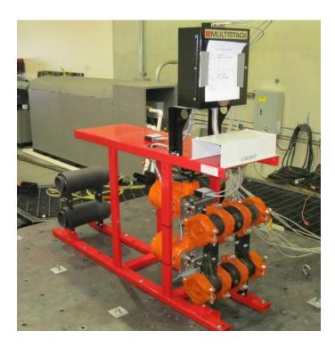
The unit was mounted to the DCL shake table interface plate with six 3/8" diameter Grade 5 bolts.
