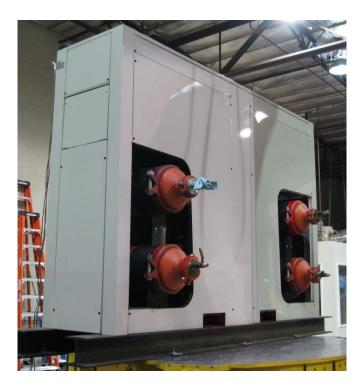
The unit was mounted to the DCL shake table interface frame with four 1/2" diameter Grade 5 bolts.
