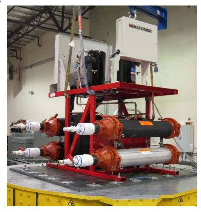
The unit was mounted to the DCL shake table interface plate with six 1/2" diameter A307 bolts.
