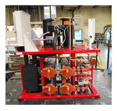
The unit was flexibly base mounted with six 3/8" thick, 4"x4" rubber pads (Bramec model 6434) and six 1/2" diameter Grade 5 bolts.
