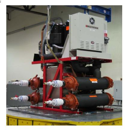
The unit was mounted to the DCL shake table interface plate with six 1/2" diameter A307 bolts.
