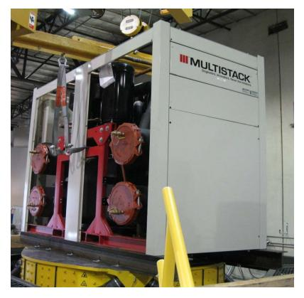
The unit was mounted to the DCL shake table interface frame with six 3/4" diameter A307 bolts.
