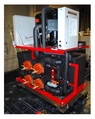
The unit arrived at DCL pre-mounted to a steel lifting frame with four 1/2" diameter Grade 5 bolts. The lifting frame was attached to four isolators (VMC model MSH-1E-825N) with one 5/8" diameter Grade 5 bolt per isolator. Each isolator was attached to the shake table interface plate with four 1/2" diameter Grade 5 bolts.
