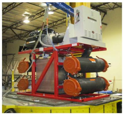
The unit was mounted to the DCL shake table interface plate with six 5/8" diameter A307 bolts.
