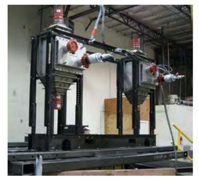
All units were filled with contents and maintained structural integrity and functionality after shake table test
