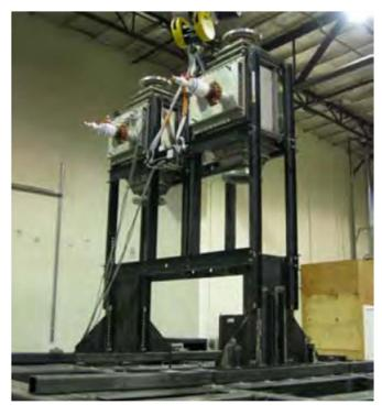
All units were filled with contents and maintained structural integrity and functionality after shake table test
