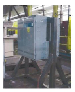
The UUT was mounted to a wall mounting fixture using (6) 3/8" Grade 5 bolts. Unit maintained structural integrity and remained functional per manufacturer requirement. Contents were included in testing per operating conditions.
