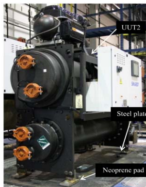
Figure 2- UUT-2 Test Configuration
