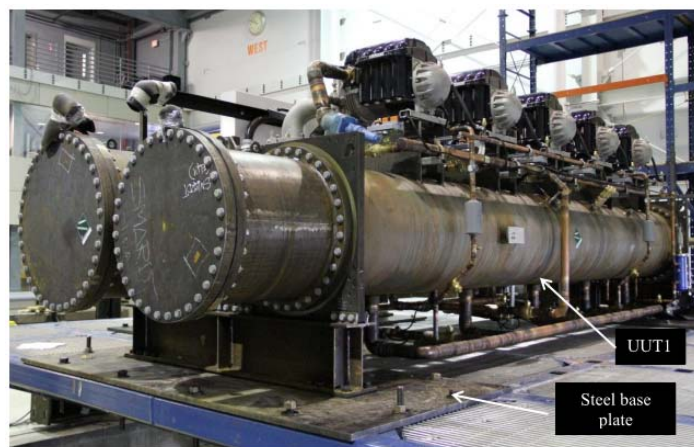
Figure 1 – UUT-1 Test Configuration
