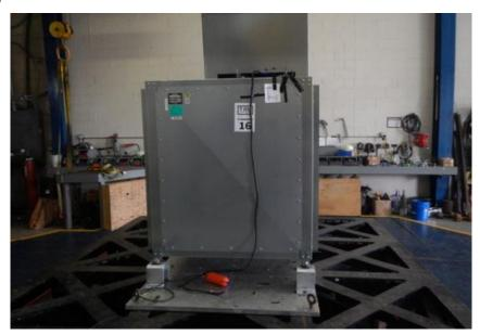
Floor mounted - isolated using (4) SRS-450 isolators w/ (1) 5/8" Grade 8 bolt attaching Isolator to unit & (2) 5/8" Grade 8 bolts attaching each isolator to the table.
