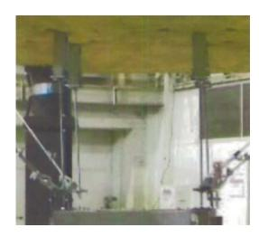
Ceiling mounted - isolated using Caldyne HH30 ET80 isolators and 1/4" diameter carbon steel cables. 3/8" ASTM A307 Grade A steel threaded rods connected to UUT through (2) 1/4" thick angle brackets fastened using (1) 5/16" Grade 2 bolt and bolted together with (2) 3/8" Grade 5 bolts. Unit maintained structural integrity and remained functional per manufacturer requirement after shake table test. Contents were included in testing per operating conditions.
