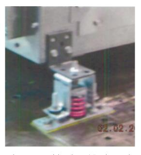
Floor mounted - isolated using Caldyne JQBKS-ET473 isolators. Isolators mounted directly to 1/4" carbon steel angle brackets which are attached to the side of the UUT at the base using (2) 5/16" Grade 2 bolts. Each isolator was attached to the table using (2) 1/2" Grade 5 bolts. Unit maintained structural integrity and remained functional per manufacturer requirement after shake table test. Contents were included in testing per operating conditions.
