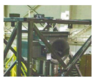
Ceiling mounted - isolated using Caldyne HH30-ET940 isolators. The UUT was connected to the isolators using 24" long 3/4" ASTM A307 Grade A threaded rod and 3/8" carbon steel cable at each corner. Field installations require 2 cable restraints at each corner and compression struts on each hanging rod. Unit maintained structural integrity and remained functional per manufacturer requirement after shake table test. Contents were included in testing per operating conditions.
