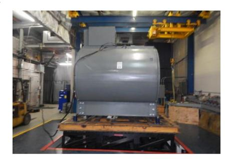
Floor mounted - isolated using (4) Mason SSLFH-C-1750 isolators w/ (1) 1/2" Grade 8 bolt attaching Isolator to unit & (4) 5/8" Grade 8 bolts attaching each isolator to the table.
