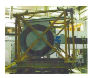
Ceiling mounted - isolated using Caldyne HH30-ET2060 isolators. The UUT was connected to the isolators using 24" long 1" ASTM A307 Grade A threaded rod with 3/8" carbon steel cable at each corner. Field installations require 2 cable restraints at each corner. Unit maintained structural integrity and remained functional per manufacturer requirement after shake table test. Contents were included in testing per operating conditions.
