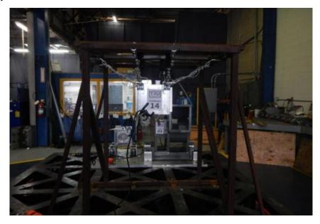
Ceiling suspended - isolated using Kinetics SH-1-70 spring isolators with (4) 18" long by 3/8" ASTM A307 Grade A threaded drop rods and (8) KSWC-2 cable braces.
