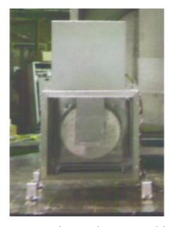
Floor mounted - isolated using Caldyne JQAE106K isolators. Isolators mounted directly to 1/4" carbon steel angle brackets which are attached to the side of the UUT at the base using (1) 5/16" Grade 2 bolt. Each isolator was attached to the table using (2) 1/2" Grade 5 bolts. Unit maintained structural integrity and remained functional per manufacturer requirement after shake table test. Contents were included in testing per operating conditions.
