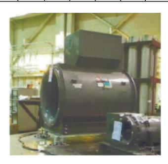
Floor mounted - isolated using a Caldyne JQBET473K isolator at each corner. Each isolator was attached to the table using (2) 1/2" Grade 5 bolts.
