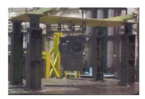
Ceiling mounted - isolated using Caldyne HH30-ET129 isolators. The UUT was attached to the isolators using 20" long 3/8" ASTM A307 Grade A threaded rod and 1/4" carbon steel cable at each corner. Field installations require 2 cable restraints at each corner and compression struts on each hanging rod. Unit maintained structural integrity and remained functional per manufacturer requirement after shake table test. Contents were included in testing per operating conditions.
