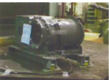
Floor mounted - isolated using JQAE106K isolators at each corner. Each isolator was attached to the table using (2) 1/2" Grade 5 bolts.
