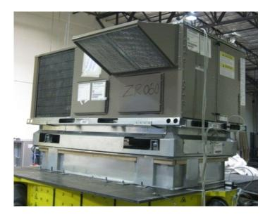
UUT4b was tested on an isolated roof curb by ProVent. The curb had four 12-gage anchoring pockets, two on each long side of the curb. The unit was attached to each of the pockets using four #12 1-1/2-inch TEK screws. The curb was attached to the 3/4-inch thick steel shake table interface plate with six 1/2-inch diameter Grade 5 bolts, one centered at each corner and one centered on each of the long sides of the curb.
