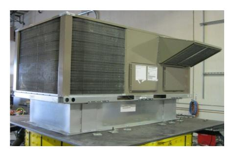
UUT4a was tested on a rigid roof curb by MicroMetl. The curb had six 10-gage anchoring pockets, three on each long side of the curb. The unit was attached to each of the pockets using four #12 1-1/2-inch TEK screws. The curb was attached to the 3/4-inch thick steel shake table interface plate with sixteen 1/2-inch diameter Grade 5 bolts, six on each long side of the curb and four on each short side, with each side sharing a bolt on the corners.
