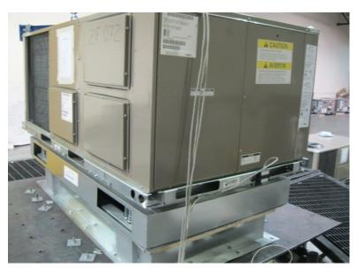
UUT6b was tested on an isolated roof curb by MicroMetl. The curb had six 10-gage anchoring pockets, three on each long side of the curb. The unit was attached to each of the pockets using four #12 1-1/2-inch TEK screws. The curb was attached to the 3/4-inch thick steel shake table interface plate with sixteen 1/2-inch diameter Grade 5 bolts, six each long side and four each short side, with each side sharing a bolt on the corners.
