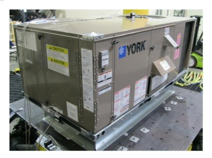
UUT5a was tested on a rigid roof curb by Ruskin. The curb had eight 10-gage anchoring pockets, three on each long side of the curb and one on each short side. The unit was attached to each of the pockets using two #14-24 x 5-inch self-drilling screws. The curb was attached to the 3/4-inch thick steel shake table interface plate with eight 3/8-inch diameter Grade 5 bolts, two on each side of the curb, each 5-inches in from the corners.
