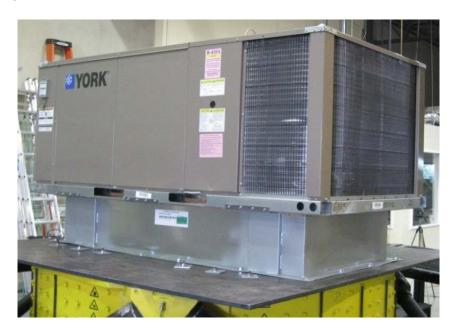
UUT1a was tested on a rigid roof curb by MicroMetl. The curb had six 10-gage anchoring pockets, three on each long side of the curb. The unit was attached to each of the pockets using four #12 1-1/2-inch TEK screws. The curb was attached to the 3/4-inch thick steel shake table interface plate with sixteen 1/2-inch diameter Grade 5 bolts, six on each long side of the curb and four on each short side, with each side sharing a bolt on the corners.
