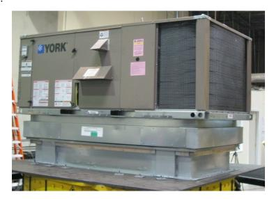
UUT5b was tested on an isolated roof curb by MicroMetl. The curb had six 10-gage anchoring pockets, three on each long side of the curb. The unit was attached to each of the pockets using four #12 1-1/2-inch TEK screws. The curb was attached to the 3/4-inch thick steel shake table interface plate with sixteen 1/2-inch diameter Grade 5 bolts, six each long side and four each short side, with each side sharing a bolt on the corners.
