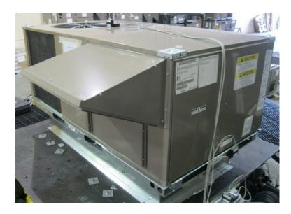
UUT3a was tested on a rigid roof curb by Ruskin. The curb had eight 10-gage anchoring pockets, three on each long side of the curb and one on each short side. The unit was attached to each of the pockets using two #14-24 x 5-inch self drilling screws. The curb was attached to the 3/4-inch thick steel shake table interface plate with eight 3/8-inch diameter Grade 5 bolts, two on each side of the curb, each 5-inches in from the corners.
