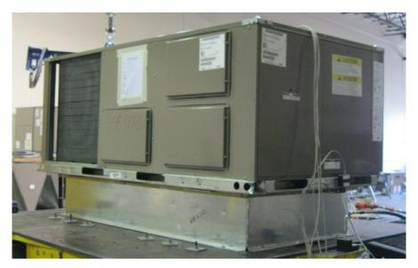
UUT6a was tested on a rigid roof curb by Ruskin. The curb had eight 10-gage anchoring pockets, three on each long side of the curb and one on each short side. The unit was attached to each of the pockets using two #14-24 x 5-inch self drilling screws. The curb was attached to the 3/4-inch thick steel shake table interface plate with eight 3/8-inch diameter Grade 5 bolts, two on each side of the curb, each 5-inches in from the corners.
