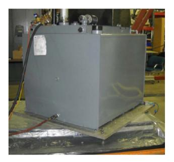
Component maintained structural integrity and functionality after shake table tests.
