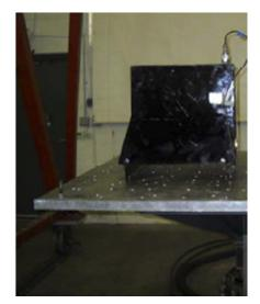
Component maintained structural integrity and functionality after shake table tests.
