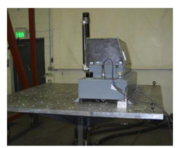
Component maintained structural integrity and functionality after shake table tests.
