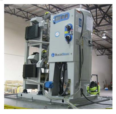
Unit base-mounted to the DCL steel shake table interface plate with four 1/2-inch diameter Grade 5 bolts. The plate was attached to the shake table with M12 threaded rod, spaced approximately 8-inches on-center.
