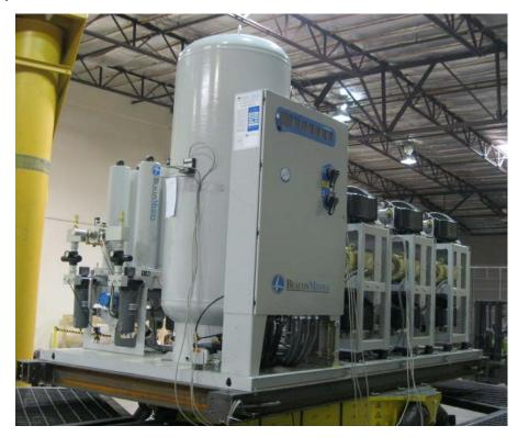
Unit base-mounted to the DCL steel shake table interface fixture with sixteen 1/2-inch diameter Grade 5 bolts. The fixture was attached to the shake table with M12 threaded rod, spaced approximately 8-inches on-center.
