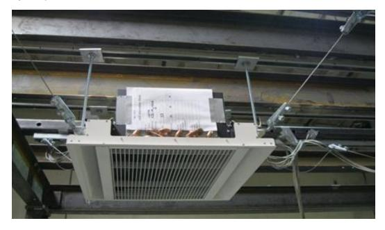
Unit was ceiling-suspended from the DCL shake table interface frame using 3/8-inch diameter threaded rod (12-inch length between attachment points), SCBH Mason brackets, 1/8-inch diameter steel cable and four manufacturer-provided friction clip brackets. The rod was attached to the interface frame with strut nuts and the Mason brackets were attached to the interface frame with 1/2-inch diameter Grade 5 bolts.
