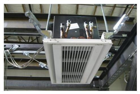
Unit was ceiling-suspended from the DCL shake table interface frame using 3/8-inch diameter threaded rod (12-inch length between attachment points), SCBH Mason brackets, 1/8-inch diameter steel cable, and four manufacturer-provided friction clip brackets. The rod was attached to the interface frame with strut nuts and the Mason brackets were attached to the interface frame with 1/2-inch diameter Grade 5 bolts.
