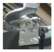
Terminal bracket used for UUT7B tests. Brackets are 12 gage zinc-coated steel attached to unit with four #14 sheet metal screws.
