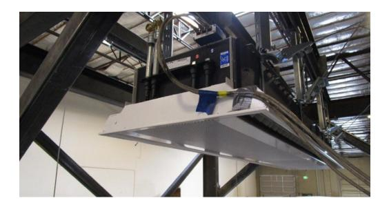
The unit was ceiling-suspended from the DCL shake table interface frame using 3/8-inch diameter threaded rod (8 pieces), spaced at a maximum of 37 inches on-center. Grade 5 nuts, 3/8-inch spring nuts and 16-inch long rod stiffeners, consisting of strut and rod stiffening clips, were used. Lateral bracing consisted of 8 SCB1 and SCBH1 brackets and 3/16 inch diameter steel cable. The unit was suspended approximately 18 inches from the top of the shake table interface frame.
