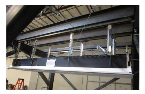
The unit was ceiling-suspended from the DCL shake table interface frame using 3/8-inch diameter threaded rod (8 pieces), spaced at a maximum of 37 inches on-center. Grade 5 nuts, 3/8-inch spring nuts and 16-inch long rod stiffeners, consisting of strut and rod stiffening clips, were used. Lateral bracing consisted of 8 SCB1 and SCBH1 brackets and 3/16 inch diameter steel cable. The unit was suspended approximately 18 inches from the top of the shake table interface frame.
