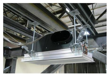
Unit was ceiling-suspended from the DCL shake table interface frame using 3/8-inch diameter threaded rod (12-inch length between attachment points), SCBH Mason brackets, 1/8-inch diameter steel cable, and four manufacturer-provided friction clip brackets. The rod was attached to the interface frame with strut nuts and the Mason brackets were attached to the interface frame with 1/2-inch diameter Grade 5 bolts.
