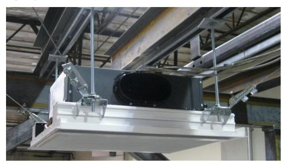
Unit was ceiling-suspended from the DCL shake table interface frame using 3/8-inch diameter threaded rod (12-inch length between attachment points), SCBH Mason brackets, 1/8-inch diameter steel cable and four manufacturer-provided friction clip brackets. The rod was attached to the interface frame with strut nuts and the Mason brackets were attached to the interface frame with 1/2-inch diameter Grade 5 bolts.
