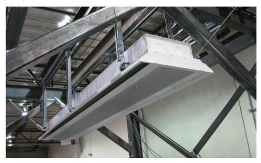
Unit was ceiling-suspended from the DCL shake table interface frame using 3/8-inch diameter threaded rod, SCBH Mason brackets, 3/16-inch diameter steel cable, and six manufacturer-provided friction clip brackets. The threaded rod was stiffened with slotted A-12 channed and rod stiffening clips spaced at approximately 10-inches on-center. The rod was attached to the interface frame with strut nuts and the Mason brackets were attached to the interface frame with 1/2-inch diameter Grade 5 bolts.
