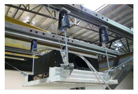
Unit was ceiling-suspended (with spring isolators) from the DCL shake table interface frame using 3/8-inch diameter threaded rod (12-inch length between attachment points), SCBH Mason brackets, 1/8-inch diameter steel cable and four manufacturer-provided friction clip brackets. The rod was attached to Mason RW30N-B-138 spring isolators, which were in turn attached to the interface frame with strut nuts. The Mason brackets were attached to the interface frame with 1/2-inch diameter Grade 5 bolts.
