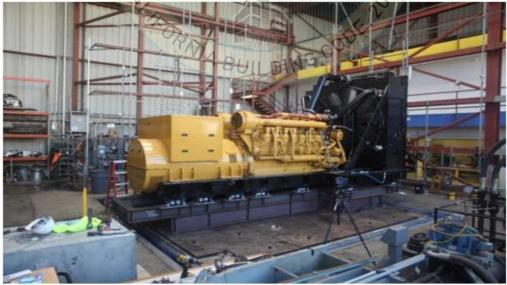
Unit is mounted to test fixture using (14) VMC M2SSH-1E 5150 spring isolators (and included hardware). The isolators were welded to the test fixture using (3) 1" long 5/16" fillet welds along the long sides, and a 5/16" fillet weld along the entire length of the short sides.
