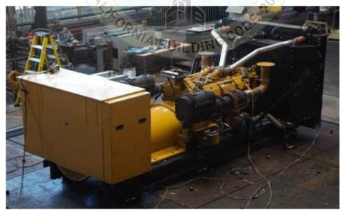
Unit is mounted to test fixture using (6) VMC M2SSH-1E 5150 spring isolators (and included hardware). (12) 3/4" Grade 8 bolts are used to mount the isolators to the test fixture.
