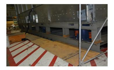
**Unit-to-Unit Fixture:** (16) 5/8" A325 bolts; For rigid base mounting, the isolators are locked through blocking at fixtures. Unit maintained structural integrity and remained functional per manufacturer requirement. Contents were included in testing per operating conditions.
