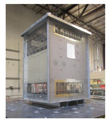
Unit was rigidly attached to shake table interface frame with (4) 1/2" diameter Grade 5 bolts
