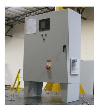
The unit was mounted to the DCL shake table interface plate with eight 1/2-inch diameter Grade 5 bolts.
