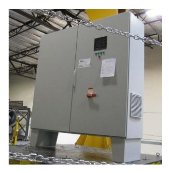
The unit was mounted to the DCL shake table interface plate with four 1/2-inch diameter Grade 5 bolts.
