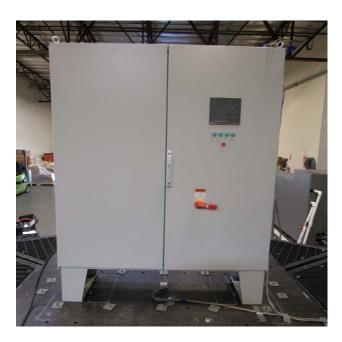
The unit was mounted to the DCL shake table interface plate with four 1/2-inch diameter Grade 5 bolts and 2-inch square 1/4-inch thick plate washers.
