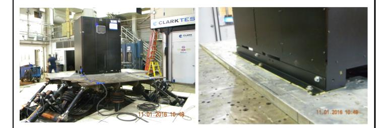
The unit was rigid floor mounted using (6) 1/2" Grade 5 bolts. Unit maintained structural integrity and remained functional per manufacturer requirement after shake table test. Contents were included in testing per operating conditions.
