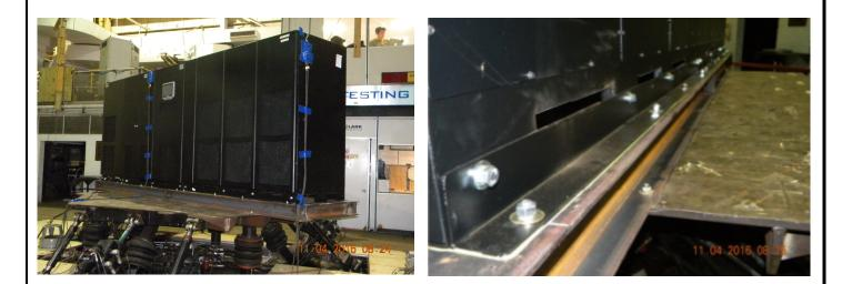
The unit was rigid floor mounted to the table using (22) 9/16" Grade 5 bolts. Unit maintained structural integrity and remained functional per manufacturer requirement after shake table test. Contents were included in testing per operating conditions.
