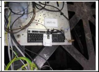
PROPERTIES: DIMENSIONS (in.) LOWEST RESONANT FREQUENCY (Hz.) Width Height Front-Axis Vert-Axis Weight (lb.) Side-Axis Depth 18 6.75 0.75 2 >50 >50 27.9 SHAKE TABLE TEST PARAMETERS CODE **TEST CRITERIA** S<sub>DS</sub> (G) z/h A<sub>FLX-H</sub> (G) A<sub>RIG-H</sub> (G) A<sub>FLX-V</sub> (G) A<sub>RIG-V</sub> (G)  $I_P$ 2.0 **CBC 2016** ICC-ES AC156 1.5 3.20 2.40 1.68 0.68 2.5 0
