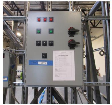
All units were filled with contents and maintained structural integrity and functionality after shake table test
