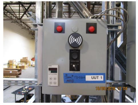
All units were filled with contents and maintained structural integrity and functionality after shake table test
