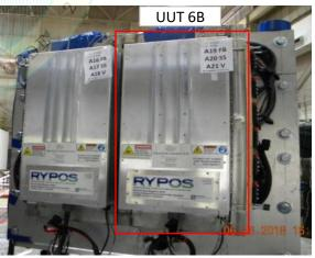
UUT 6B was installed onto a mounting frame and secured to the test fixture with sixteen (16) 5/16"-18 Grade 8 bolts, washers, and lock washers. The fixture was mounted base-rigid to the shake table with four (4) 1"-8 bolts, torqued to 220 ft-lbs. Unit maintained structural integrity and remained functional per manufacturer requirement after shake table test. Contents were included in testing per operating conditions.
