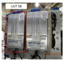
UUT 5B was installed onto a mounting frame and secured to the test fixture with sixteen (16) 5/16"-18 Grade 8 bolts, washers, and lock washers. The fixture was mounted base-rigid to the shake table with four (4) 1"-8 bolts, torqued to 220 ft-lbs. Unit maintained structural integrity and remained functional per manufacturer requirement after shake table test. Contents were included in testing per operating conditions.
