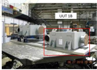
UUT 1B was installed in a test housing that was base mounted-rigid to the shake table with four (4) 1"-8 Grade 5 bolts with lock and flat washers.
