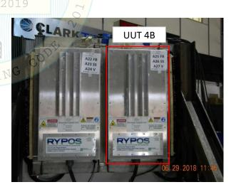
UUT 4B was installed onto a mounting frame and secured to the test fixture with sixteen (16) 5/16"-18 Grade 8 bolts, washers, and lock washers. The fixture was mounted base-rigid to the shake table with four (4) 1"-8 bolts, torqued to 220 ft-lbs. Unit maintained structural integrity and remained functional per manufacturer requirement after shake table test. Contents were included in testing per operating conditions.
