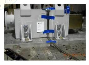
UUT 2B was installed in a test housing that was base mounted-rigid to the shake table with four (4) 1"-8 Grade 5 bolts with lock and flat washers.
