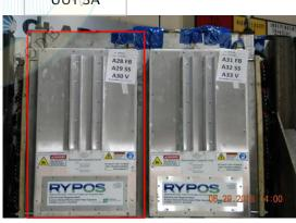
UUT 3A was installed onto a mounting frame and the secured to the test fixture with sixteen (16) 5/16"-18 Grade 8 bolts torqued to 25ft-lbs. The wall fixture was mounted with to four (4) Mason SLRSO-B-450 isolators using four (4) 1/2"-13 grade 5 bolts, washer, and lock washers. Each isolator was mounted to the shake table with four (4) 5/8"-11 grade 5 bolts with lock and flat washers, for a total of sixteen (16) 5/8"-11 grade 5 bolts.
