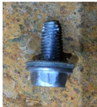
Figure UUT-3.4: Lower left front screw fell out
