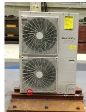
Figure UUT-3.5: Location of screw failure
