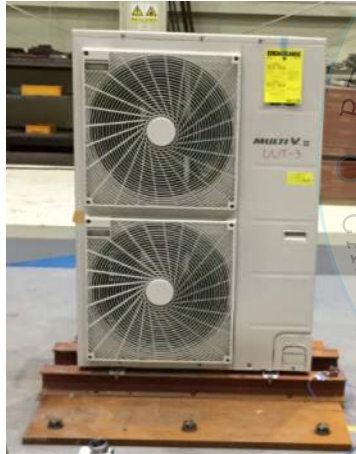
Figure UUT-3.1: Unit on the shake table
