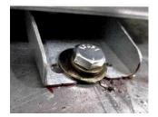
Unit mounted to the shake table with four (4) 3/8"-16 Grade 5 hex bolts with 3/8" lock washer and 3/8" flat washer. Unit maintained structural integrity and remained functional per manufacturer requirement after shake table test. Contents were included in testing per operating conditions.
