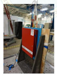
Unit mounted to wall fixture with five (5) 1/4"x 3/4" wood screws. Washers were used in addition to the wood screw at each corner.
