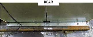
The UUT was rigid-base mounted using (2) customer provided seismic kits (PN: GVSOPT002). (16) M8 bolts and washers were used to mount the brackets to the UUT, and (15) M12 bolts were used to mount the UUT to the shake table.
