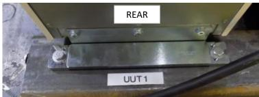
The UUT was rigid-base mounted using customer provided seismic kit (PN:GVSOPT003). (6) M8 bolts and washers were used to mount the bracket to the UUT, and (4) M12 bolts were used to mount the UUT to the shake table.
