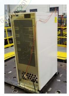
The UUT was rigid-base mounted using customer provided seismic kit (PN: GVSOPT002). The seismic kit mounting details can be found on the following page. M8 bolts were torqued to 21 Nm. M10 bolts were torqued to 42 Nm.
