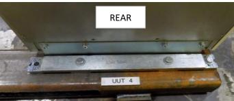
The UUT was rigid-base mounted using customer provided seismic kit (PN:GVSOPT002). (8) M8 bolts and washers were used to mount the bracket to the UUT, and (8) M12 bolts were used to mount the UUT to the shake table.
