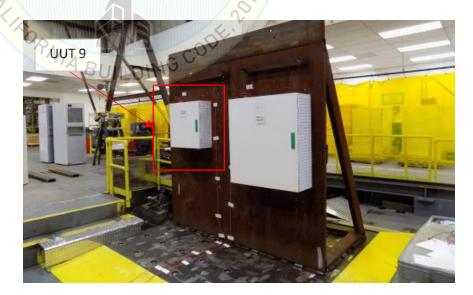
The UUT was wall mounted rigid using four (4) M10 8.8 bolts.
